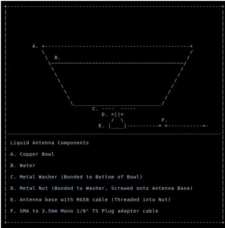
Figure 3. Liquid antenna diagram. Natan Diacon-Furtado, Community Portal , 2025. © All rights reserved, courtesy of the authors.
